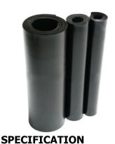
EPDM or Ethylene Propylene Diene Monomer, We highly recommended for outdoor uses as it extremely resistant to oxidation, U.V. Rays and Ozone. due to its highly saturated polymer chain. However, EPDM does not have good oil resistance like Nitrile Rubber, Is resistant to many chemicals and solvents and shows good resistance to many corrosive chemicals.
