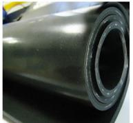
Nitrile Rubber is a copolymer of butadiene and acrylonitrile. NBR Rubber has good oil resistant performance, along with excellent abrasion and Tear Resistance, and permeability to gases.
